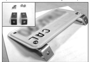
3) \*Install license plate brackets to back side of license plate as shown. Now hold license plate in desired location on undertail, carefully mark and drill holes, install using the two (2) sets of allen bolts and lock nuts.
