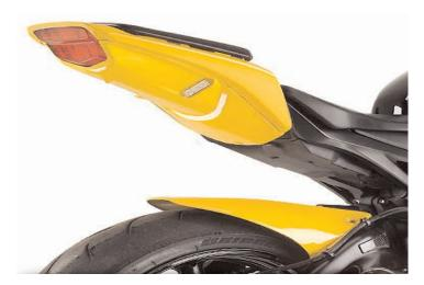
**8)** Slide undertail into tail section one side at a time, tail section should wrap around undertail and hold it securely. Phillips head screw that is provided will mount at the bottom of undertail in to well nut, from step 7. You're done!
