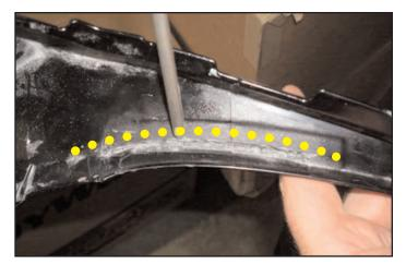
**3)** Trim inner plastic lip off of inside right and left sides of the tail section. Trim the plastic off and make the lip smooth with the surrounding plastic. You can test fit the new undertail and tail section while off the bike to ensure a good snug fit.
