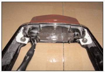
**5)** Assemble brackets to tail light and then assemble tail light to tail section making sure tail light is securely mounted.
