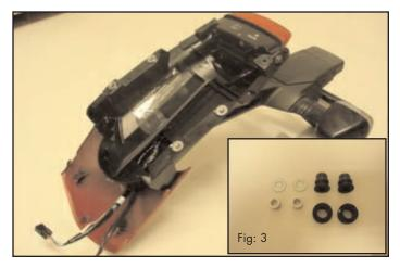
**2)** Remove tail light held on by 2 phillip screws from OEM undertail. Remove 2 well nuts and 2 rubber gromets from OEM undertail to be re-used with new undertail (as seen in Fig: 3).
