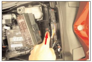
**6)** Re-install tail section, using stock hardware. Under fuse box drill out mounting hole big enough to install rubber well nut that is provided with the kit.
