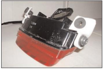
**4**) Assemble white plastic brackets (provided) with hardware from step 2; Fig: 1.
