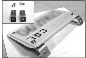
7) \*Install license plate brackets to back side of license plate as shown. Now hold license plate in desired location on undertail, carefully mark and drill holes, install using the two (2) sets of allen bolts and lock nuts.
