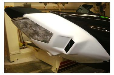
8) Align side tail section pieces with new undertail and attach all stock mounting bolts. Re-attach seat and your done! Adjust the brake light as necessary and tighten the nuts from step #7.
