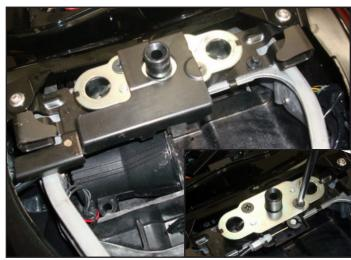
2) Remove stock undertail by removing seat latch (2 Phillips head screws), disconnect tail light. Remove undertail, lock assembly, and tail light. Save all bolts and hardware for re-installation.
