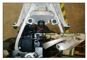
8) Attach the light to the light brackets as shown using the stock hardware, similar to the stock undertail.
