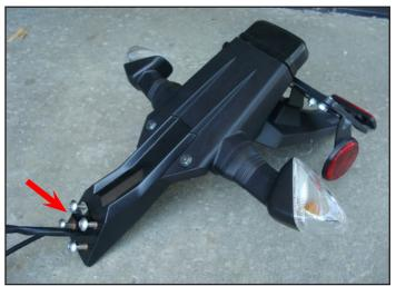
1) Remove 5mm hex bolts to undo mudflap (as pointed out) bolts are located inside glovebox. Disconnect signal light and license plate light wires to remove mudflap completely. Then remove tail section from subframe.
