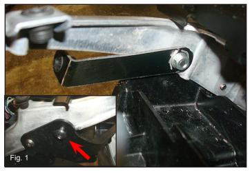
7) Replace the top bolt shown (inset) with the longer bolt provided in the kit. Attach the light brackets as shown, leave the bolt hand snug so you can adjust the light to the undertail in step 9.
