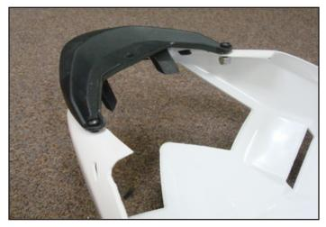
4) Attach black plastic piece that was removed (Step 3) and attach to the new undertail with provided small nuts and bolts.
