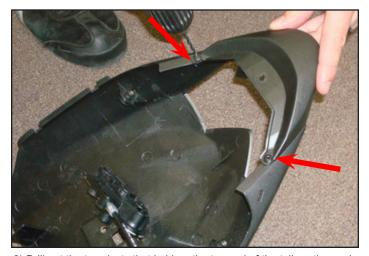
3) Drill out the two rivets that hold on the top end of the tail section and remove top piece (as shown in photo). Separated top piece will bolt on to new undertail with nuts and bolts supplied.
