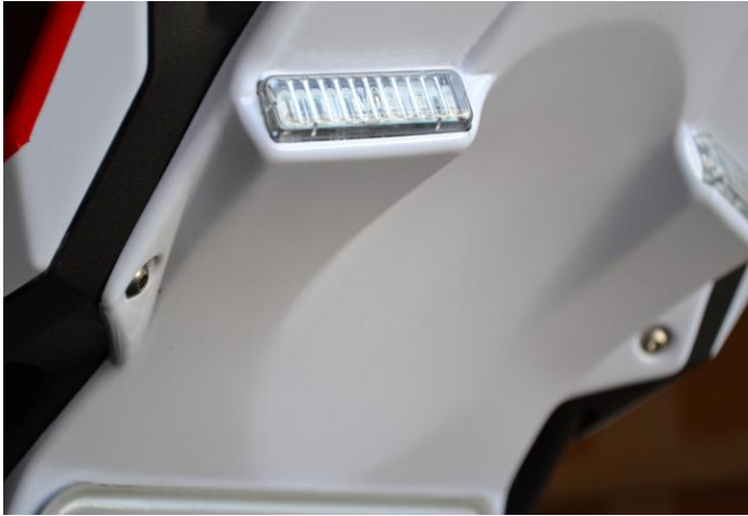
Close up of undertail corners secured to OEM body after steps 6-7 have been completed.
