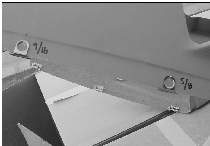
5) Measure from the lip down to the center and write the measurement on the body panel for easy reference later. Not every clip will be identical so measure each individually for perfect accuracy. Measure twice, drill once!
