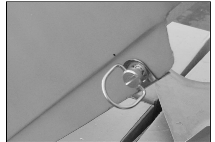
10) Check to make sure the "d-rings" fit through the body panel and clips, adjust if necessary.
