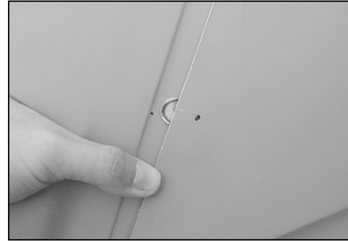
7) Place upper and lowers back together and check to make sure the marks line up, correct as necessary. Measure twice, drill once!
