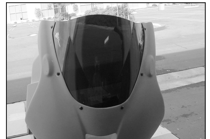
12) Mark and drill windscreen on bodywork, mount screen to upper fairing. DO NOT drill the upper fairing stay yet! Measure twice, drill once!
