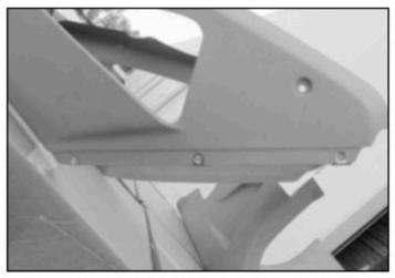
Attach the clips evenly along both sides over the recessed body panel.
