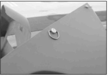
Check to make sure the "d-rings" fit through the body panel, adjust if necessary.
