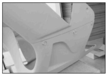
Assemble upper and lower off the bike to make sure there are no problems that need adjustments.
