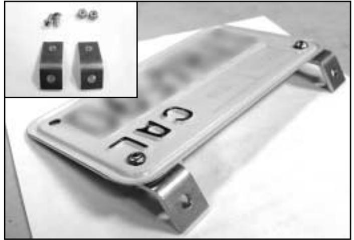
**4)** \*Install license plate brackets to back side of license plate as shown. Now hold license plate in desired location on undertail, carefully mark and drill holes, install using the two (2) sets of allen bolts and lock nuts.
