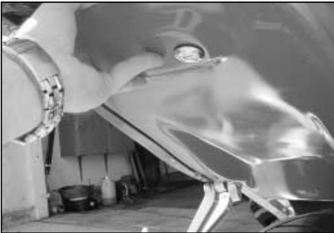
**5)** Re-mount glove box to bike using stock hardware. Replace tail section, do not use any fasteners until undertail is in place. Insert undertail left side first, then right side, be carefully not to crack or scratch undertail. Tighten light first, then all other bodywork mounting locations, then insert 2 screw rivets into stock locations into undertail.
