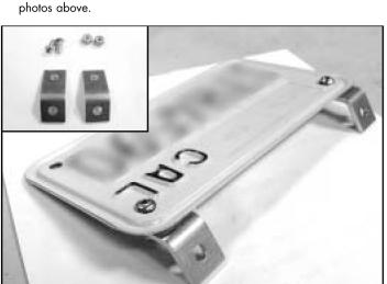
3) \*Install license plate brackets to back side of license plate as shown. Now hold license plate in desired location on undertail, carefully mark and drill holes, install using the two (2) sets of allen bolts and lock nuts.
