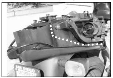
2) Using a "Dremel" tool or cutting disc, remove the plastic shown in the photos above.
