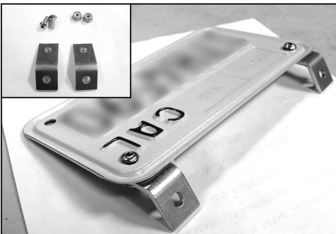
**4)** \*Install license plate brackets to back side of license plate as shown. Now hold license plate in desired location on undertail (under the signals), carefully mark and drill holes, install using the two (2) sets of bolts & nuts.
