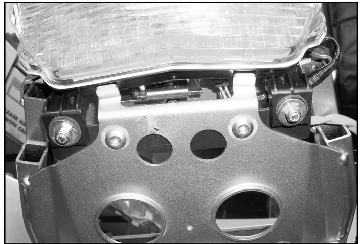
**3)** Mount the bracket/brake light inside of subframe as shown using stock hardware. Re-assemble tail, mount undertail into tail section.
