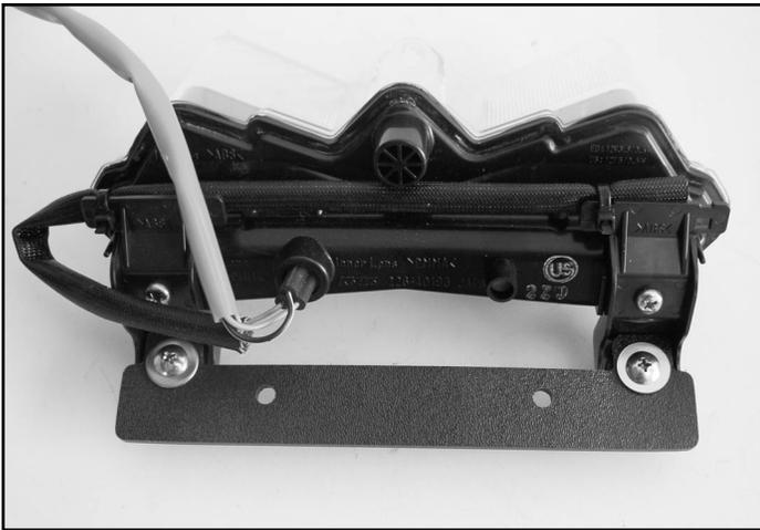
**2)** After removing the stock brake light, attach flat plastic bracket on the inside edge supplied with kit as shown using hardware provided.
