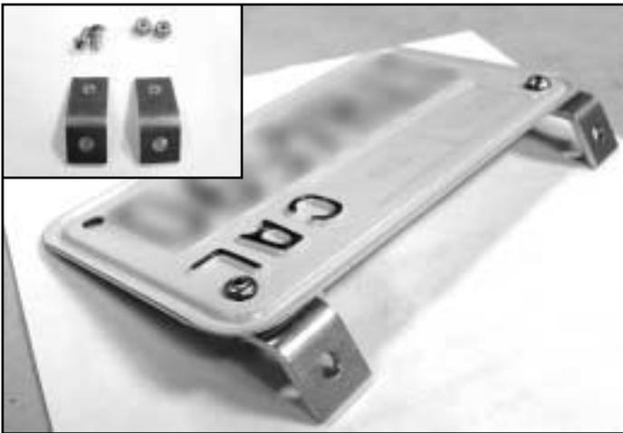
**2)** \*Install license plate brackets to back side of license plate as shown. Now hold license plate in desired location on undertail (under the signals) , carefully mark and drill holes, install using the two (2) sets of bolts & nuts.
